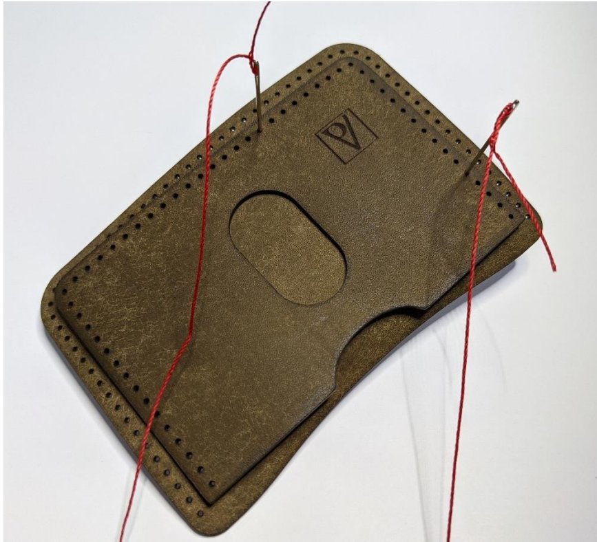
Figure 9: Needles aligning parts to be sewn.
