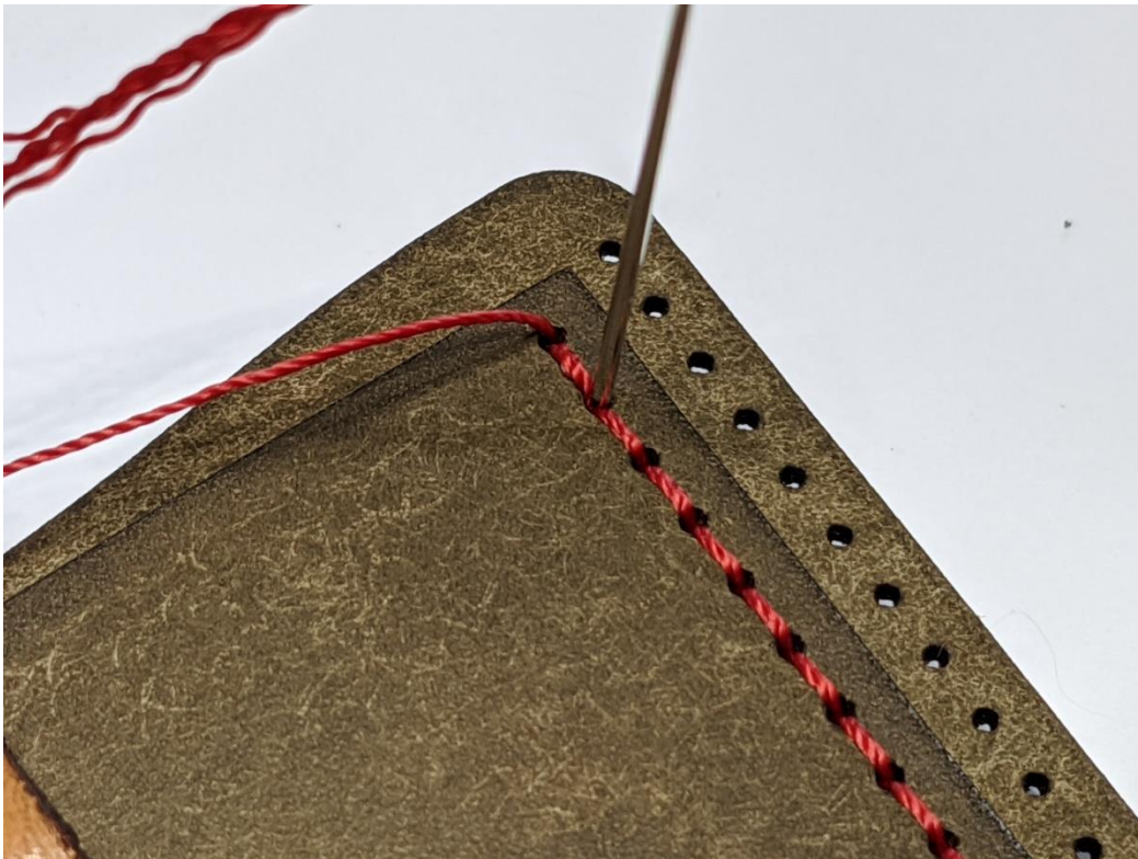
Figure 14: Back stitching to secure thread.
