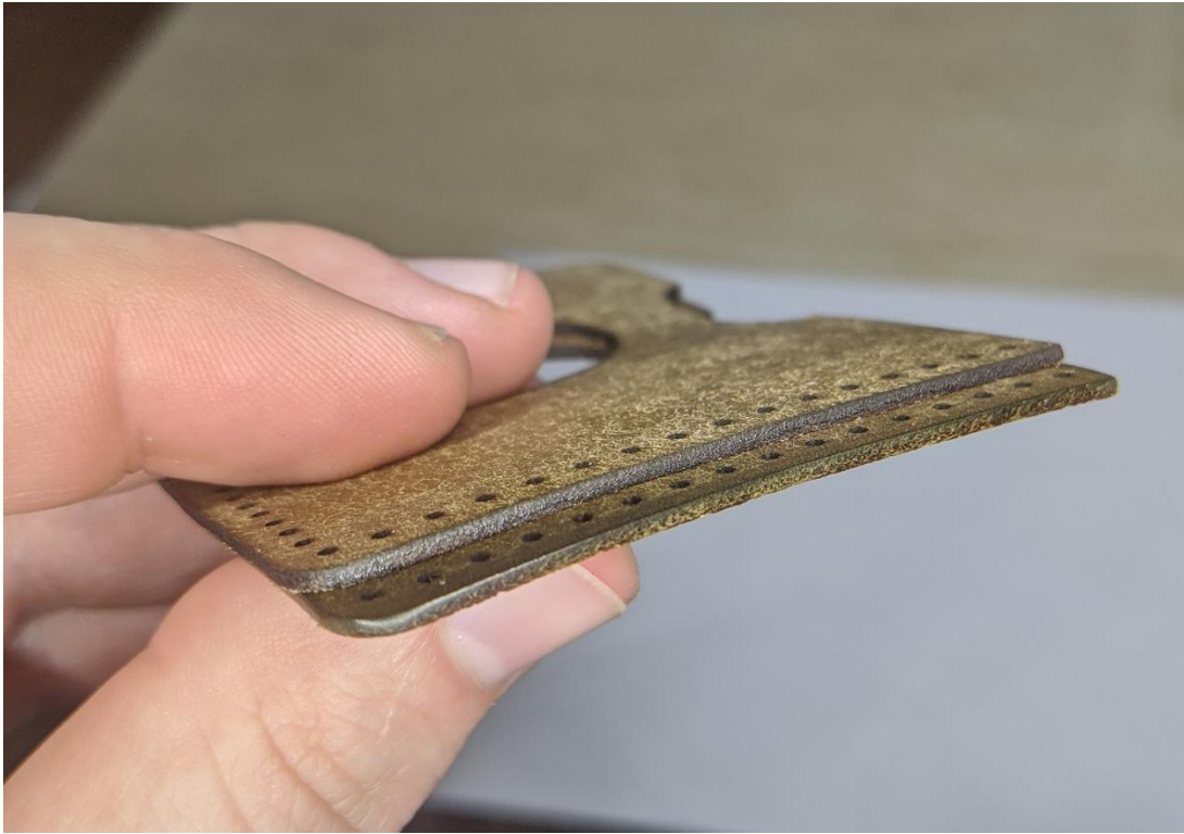
Figure 1: Edge finish options. "As Cut" shown on top, "Burnished" shown on bottom.
