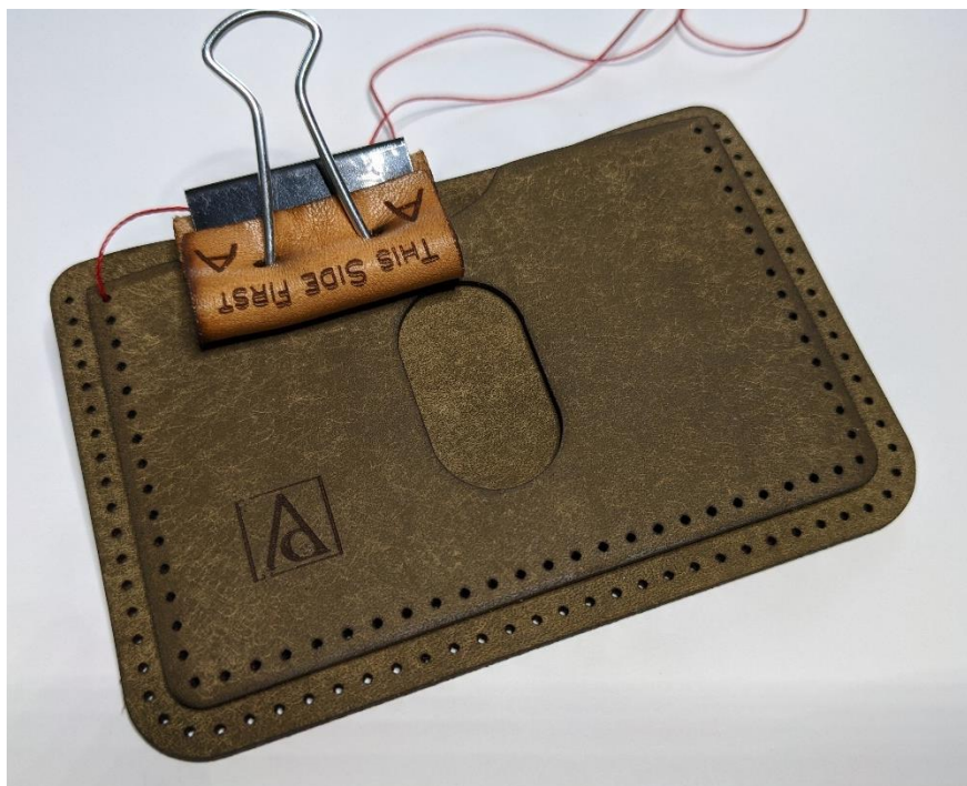
Figure 10: Clamped pieces with thread through first hole.
